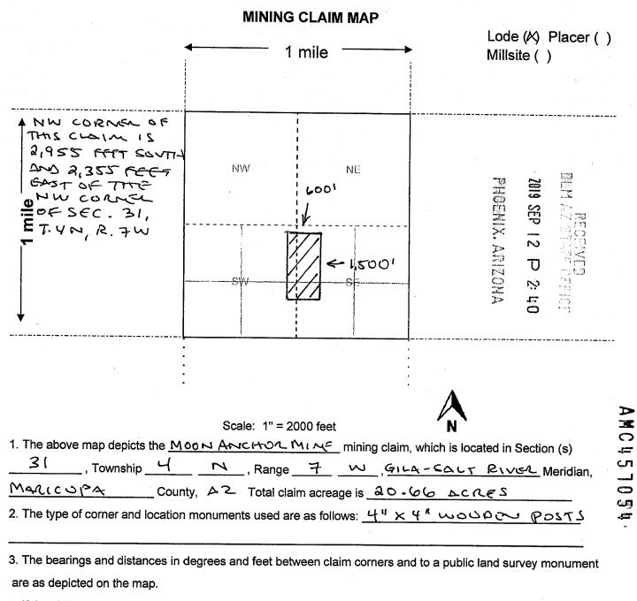
4. If the claim is a placer or millsite claim with exterior limits conforming to legal subdivisions of the public survey, provide a legal description of the claim <u>NW CURNEL OF RATS CLAIM 15 2,955</u> FEET SOUTH AND 2,355 FEET GAST FROM THE NW CURNEL OF SEC. 31, T. 4 N, R. 7 W. Form MCF100a
